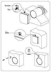
5. Install the filter, ceramic enthalpy heat exchanger, another filter and bracket inside the inner duct. In this item, carry out the step in advance in the item 3, which you have put the fittings in the inner duct
