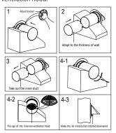
3. Install the ventilator through the wall hole from indoor, and pull back the duct by the adjust bracket to make the inner side rubber ring cling to the outside wall. Then put the inner duct in the hole and assembly inner duct and outer duct together. Fill the gap between the wall and duct with PU foam (Using waterproof sealing glue for the gap close to indoor to against rainwater). The inner duct should parallel with indoor wall surface.
