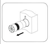
Remove the air flow rectifier and the filter in front of the regenerator.
