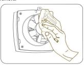
Clean the impeller blades. Use a soft brush, doth or a vacuum cleaner to clean the impeller. Do not use water abrasive detergents, solvents, sharp objects. The impeller blades must be cleaned once in year.
