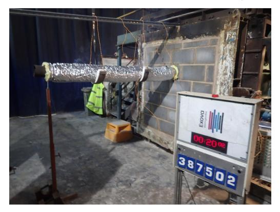
The specimen after 26 minute showing the large hole that had formed to cause integrity failure
