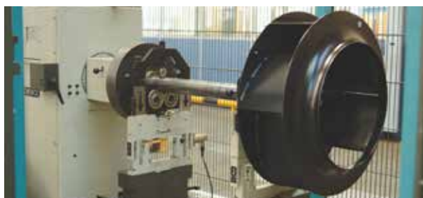
Backward curved centrifugal impellers To prevent accumulation of dirtiness. Dynamically balanced.
